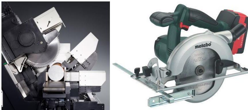
Figure 1: Spectrum of circular saw blades. Left: Machines for high output rates in mass-production (automation), Right: Battery driven handheld tool (Handcraft)
