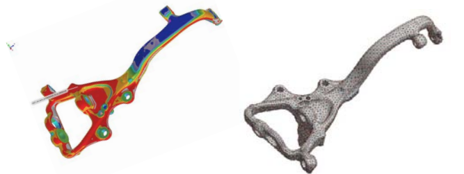
difference between measured and modeled geometry of a knuckle
