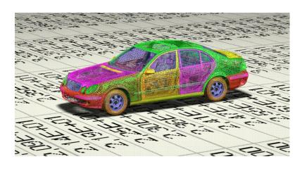
Daimler: Dr. Idrisi: "we successfully performed light weight structure optimization having up to 2000 design variables"
