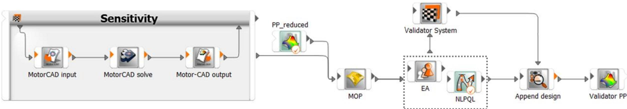
Optimization directly on the Motor-CAD system
