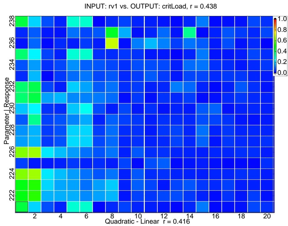
**Figure 5:** Matrix (part) of quadratic correlation coefficients. The lowest row shows correlations of the critical load with the first 20 random variables.
