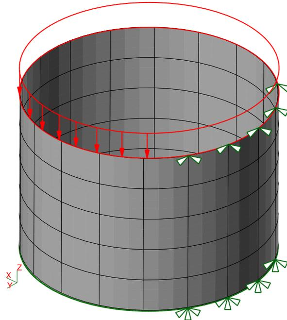
**Figure 1:** Finite element model of the cylindrical shell with schematic loads and supports.
