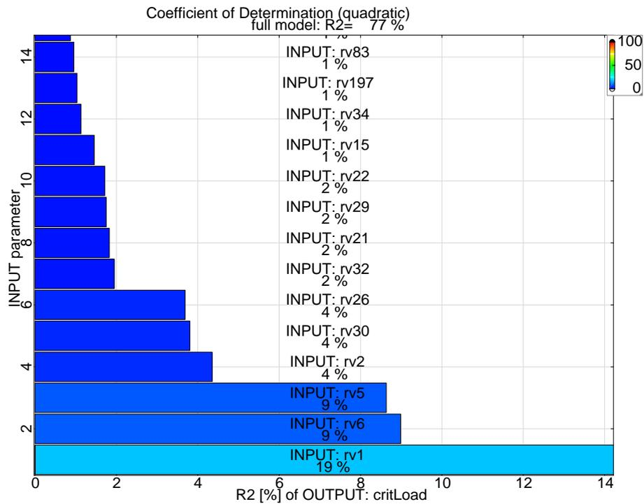
Figure 8: The top 14 coefficients of determination of critical load, quadratic regression model for random input variables.
