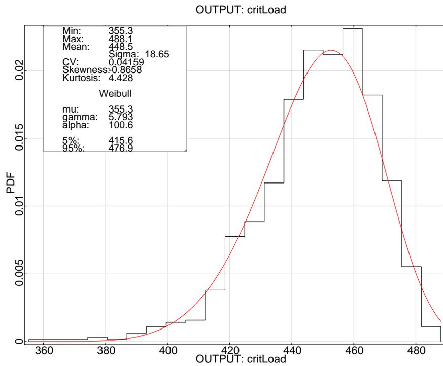
Figure 7: Histogram of the sampled critical load and fitted Weibull distribution.
