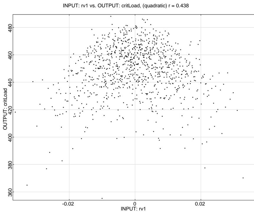
**Figure 6:** Anthill plot of critical load vs. first random variable.
