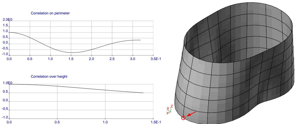
**Figure 2:** Correlation functions over perimeter (above) and height (below) and spatial correlation structure with respect to the marked node (right).
