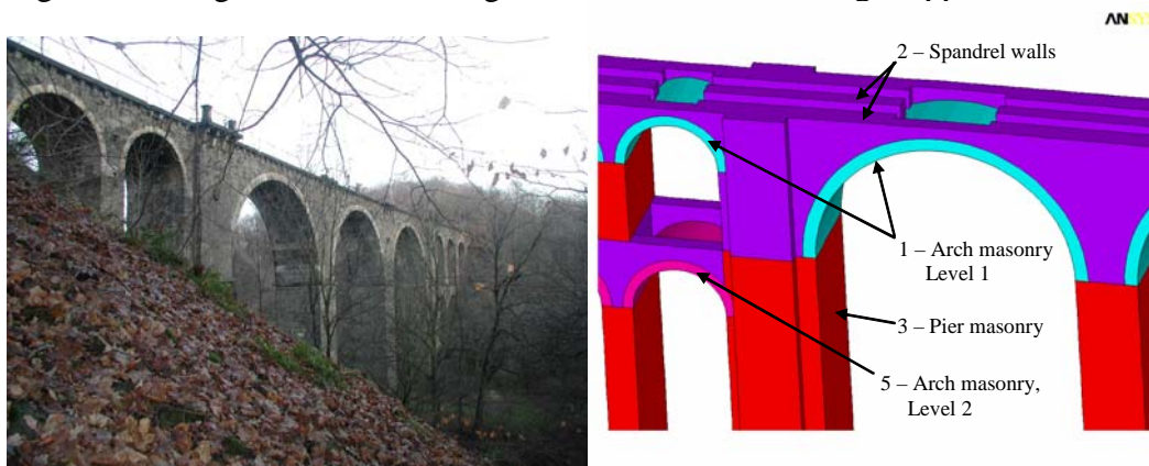
Fig. 8 Masonry arch bridge (left), material areas (right)
