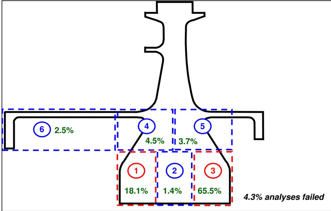
Figure 3: Partitioning of disc cross section to identify location of minimum life. Results of DOE-study: proportion that the calculated minimum life is located in the specified partitions
