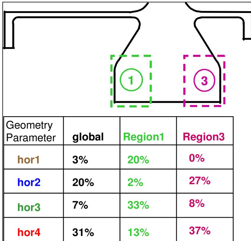
Figure 5: Results of DOE (linear coefficients of determination) considering different regions for predicted minimum life location life
