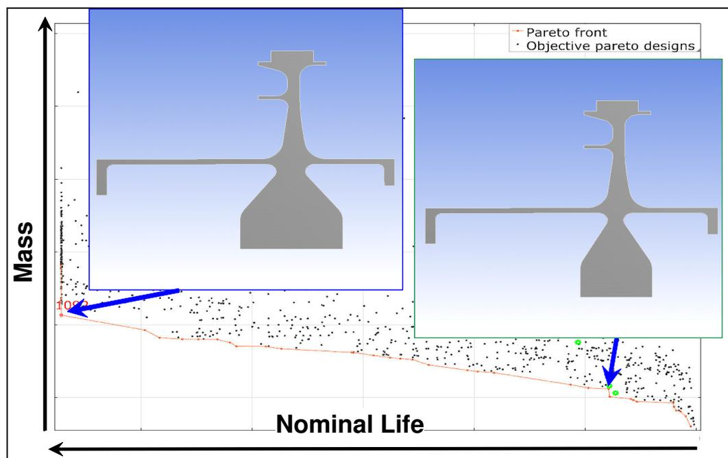
Figure 6: Result of multi-objective optimisation
