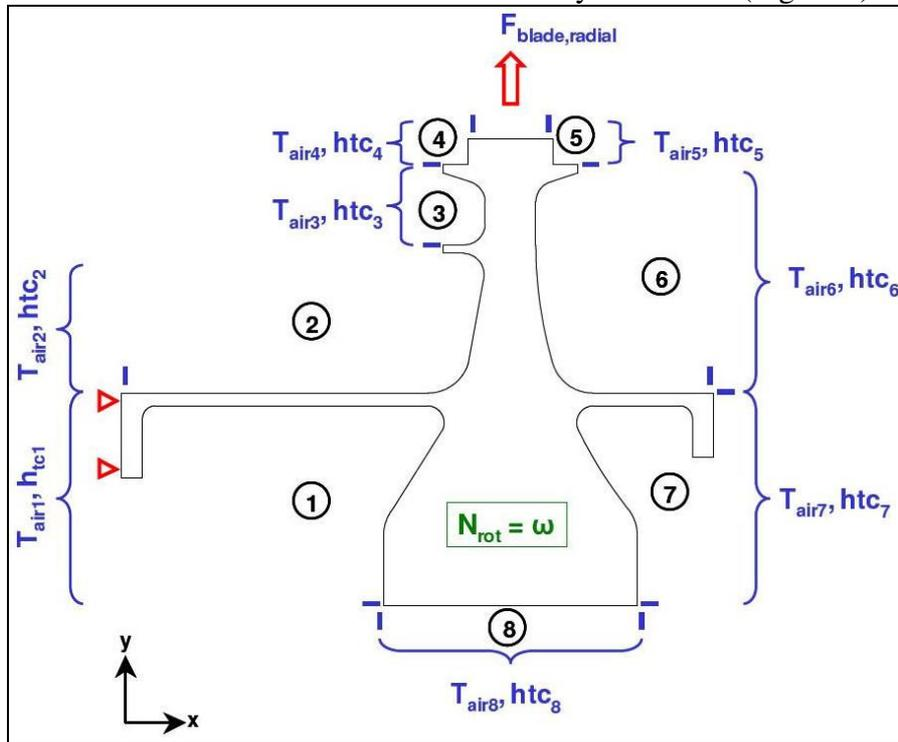
Figure 2: Axis symmetric model with schematic loads and boundary conditions
