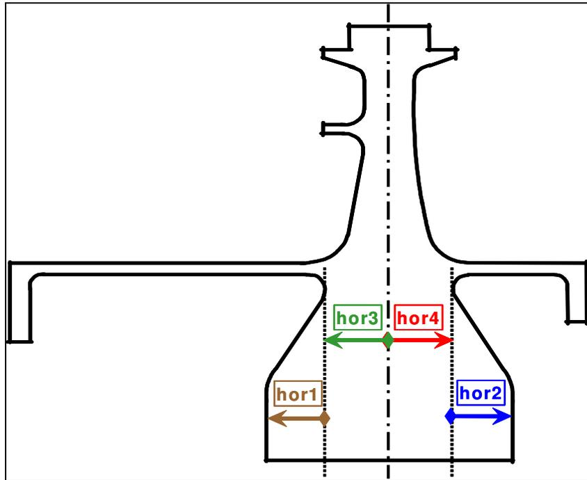
Figure 4: Illustration of the four most relevant geometry parameters as a result of the sensitivity study
