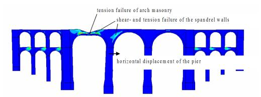
Figure 9: plastic strains and failure mechanisms
