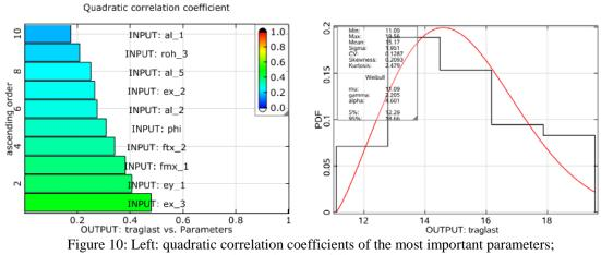
right: Histogram failure load
