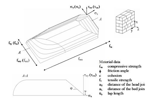
Figure 1: Yield criterion for regular masonry.
