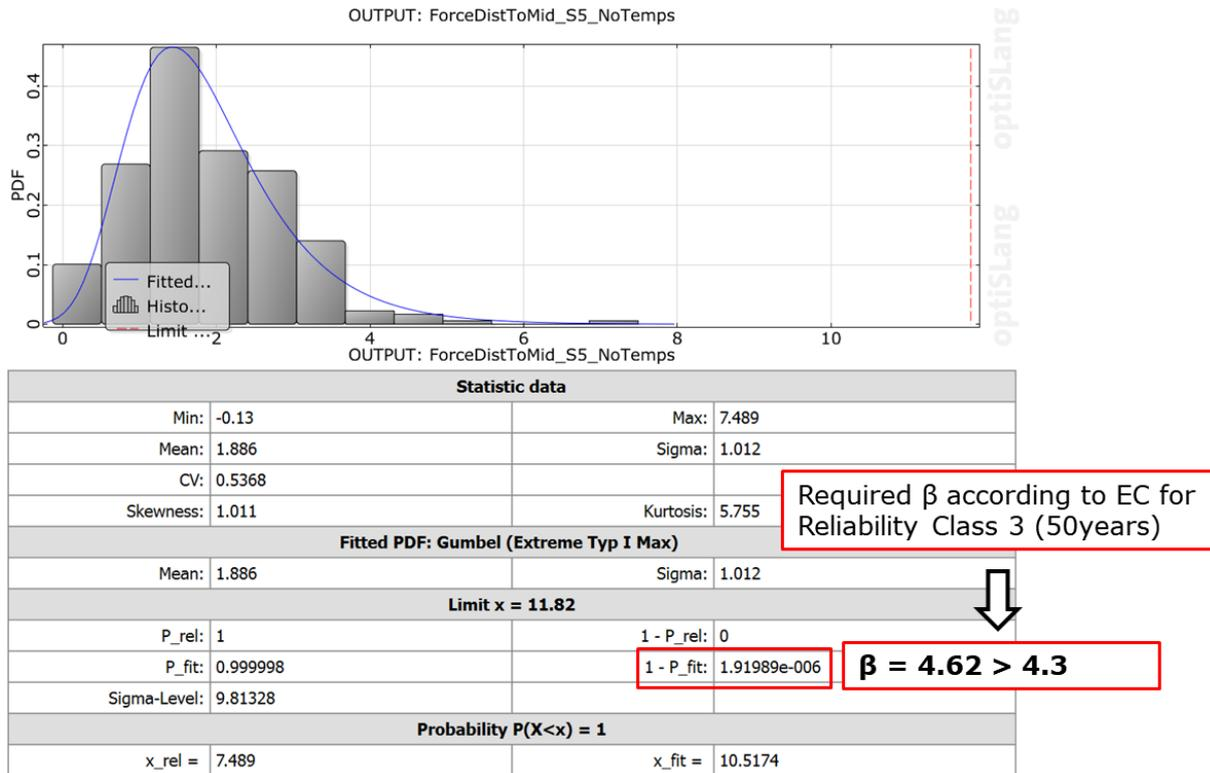
Figure 8: Calculated distribution and failure probability of the assessment criteria (here: eccentricity of the resultant force at the dam-foundation contact)
