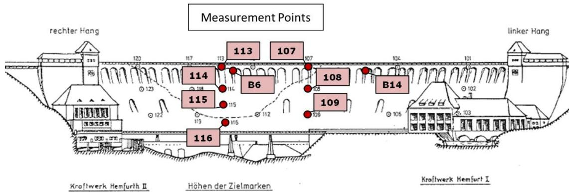
Figure 3: Displacement measurement points
