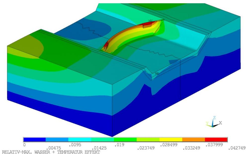
Figure 6: Load case 1 – SBS1: Displacement uSUM (m), all loads
