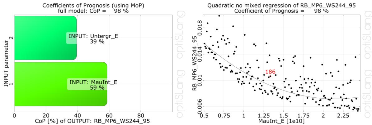
Figure 4: Results of the sensitivity analysis for measurement point B6; left: Histogram of CoP; right: Anthill-Plot of the E-modulus of the dam (MauInt\_E) vs. radial displacement at measurement point B6
