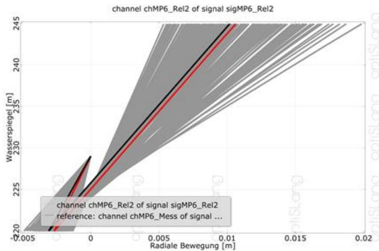
Figure 5: Radial displacement of measurement point B6, Grey: Band width of all designs; Red: Best design Nr. 186; Black: Measurement.
