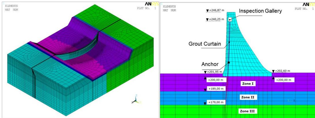
Figure 2: 3D FE-model of the dam and the dam section.
