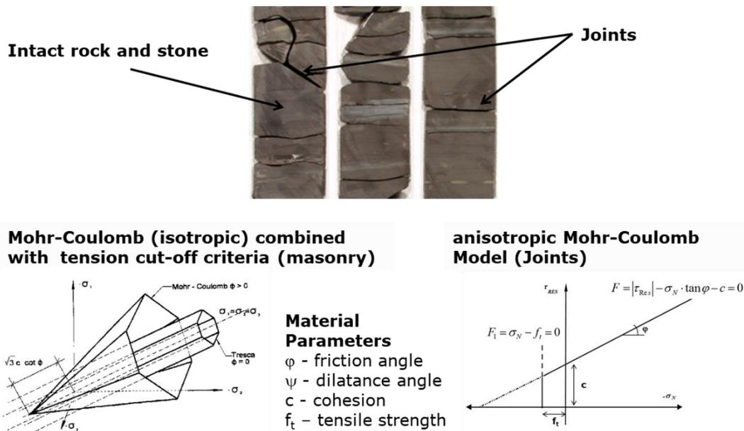
Figure 1: Constitutive models used for the masonry dam, the intact rock and the joints.
