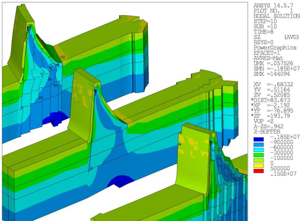
Figure 7: Load case 1 – SBS1: Vertical stresses  $\sigma_z$  (Pa), all loads
