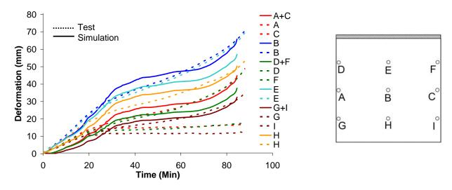
Figure 8. Wall 4 (d = 0,15 m) deformation signal – measurement versus simulation
