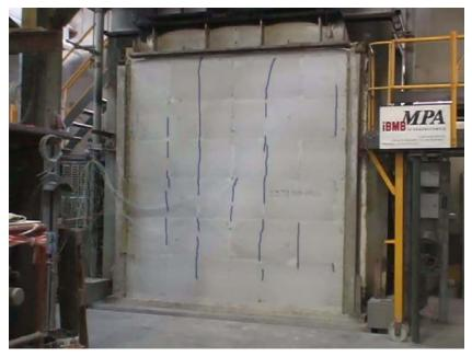
Figure 11. Observed cracking on the "cold" side, example wall 2
