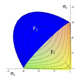
Figure 2. Modified Drucker-Prager Model for calcium silicate masonry units
