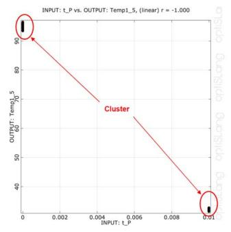
Figure 12. Anthill plot temperature in 10 mm of depth after 5 min fire loading versus thickness of plaster t\_P
