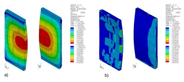
Figure 10. a) Horizontal deformations u<sub>y</sub> (m), wall 2 after 90 min, Plastic strain after 90 min, wall 2
