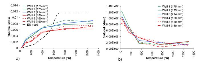
Figure 5. a) Identified curve of the thermal strain over the temperature; b) Identified curve of the young's modulus over the temperature
