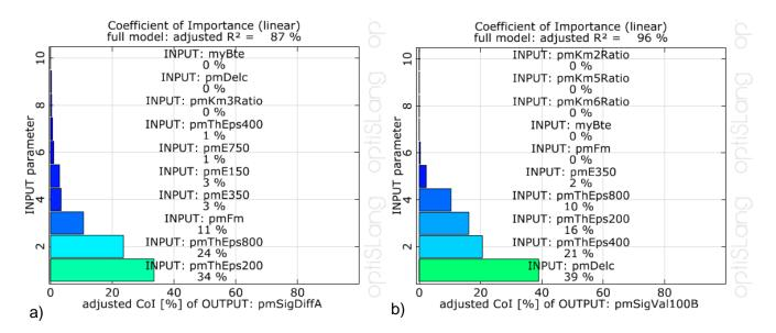
Figure 14. Coefficient of importance (CoI) of all input parameter versus deformations. a) measuring point A; b) measuring point B (measuring points A and B s. Figure 7)
