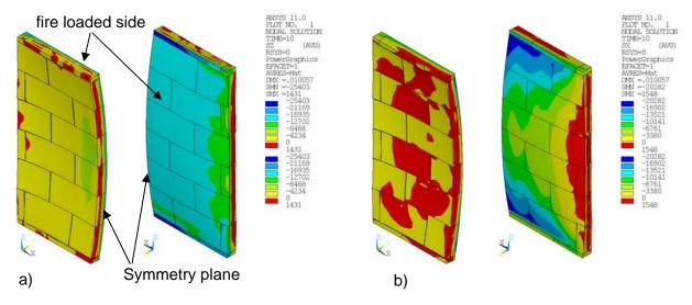
**Figure 9.** a) Typical distribution of the vertical stress in z-direction  $\sigma_z$  (kN/m<sup>2</sup>), example wall 2 b) typical distribution of the horizontal stress in x-direction  $\sigma_x$  (kN/m<sup>2</sup>), example wall 2
