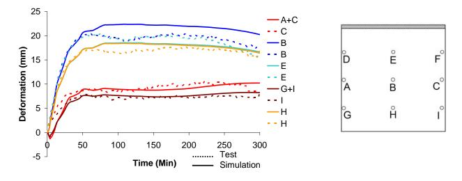
Figure 7. Wall 3 (d = 0,214 m) deformation signal – measurement versus simulation
