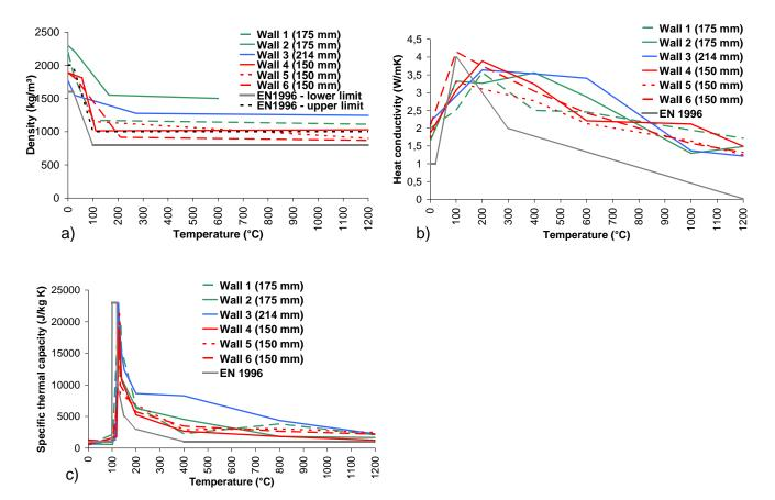
Figure 4. a) Identified curve of the density over the temperature; b) Identified curve of the heat conductivity over the temperature; c) Identified curve of the specific thermal capacity over the temperature
