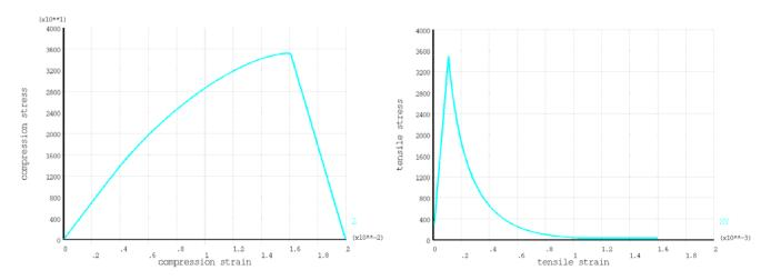
Figure 3. Stress-strain-relation: left - compression, right - tension
