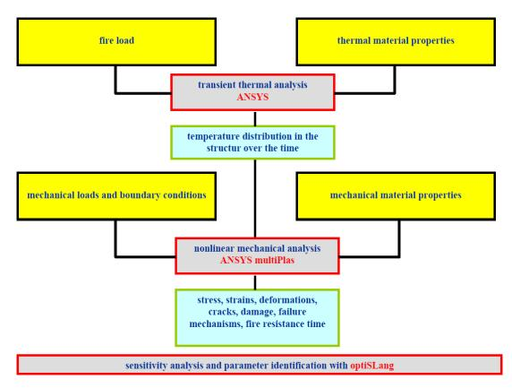
Figure 1. Simulation process
