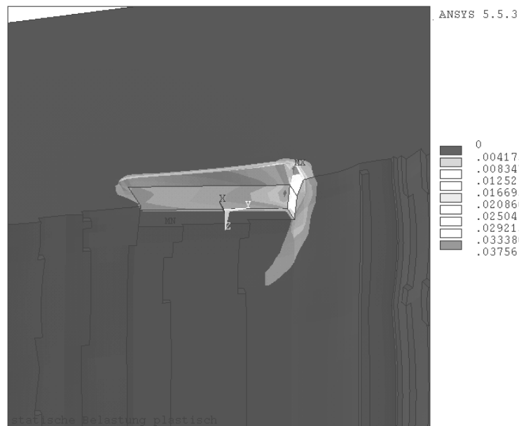
Figure 6. Plastic ground deformations during passage of two Transrapid-trains (static loading).
