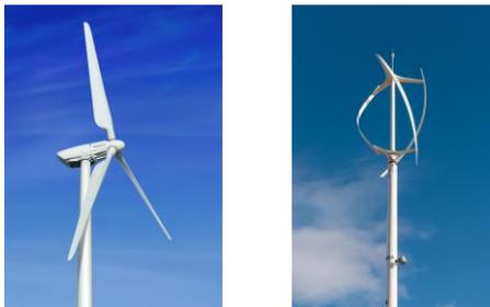
Figure 1: left - horizontal axis wind turbine (Sergiy Serdyuk – Fotolia) ; right - vertical axis wind turbine (dannyburn – Fotolia)
