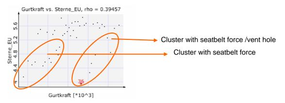
Fig. 2 Anthill plot seat belt force versus EURO NCAP evaluation. The two decreasing clusters illustrate two mechanisms of performance loss.
