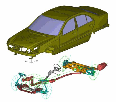
Fig. 3: Finite element vehicle model (explosion view)
