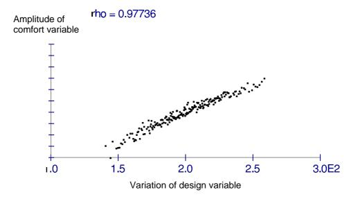
Fig. 5: Anthill plot stiffness of transmission system bearing versus response
