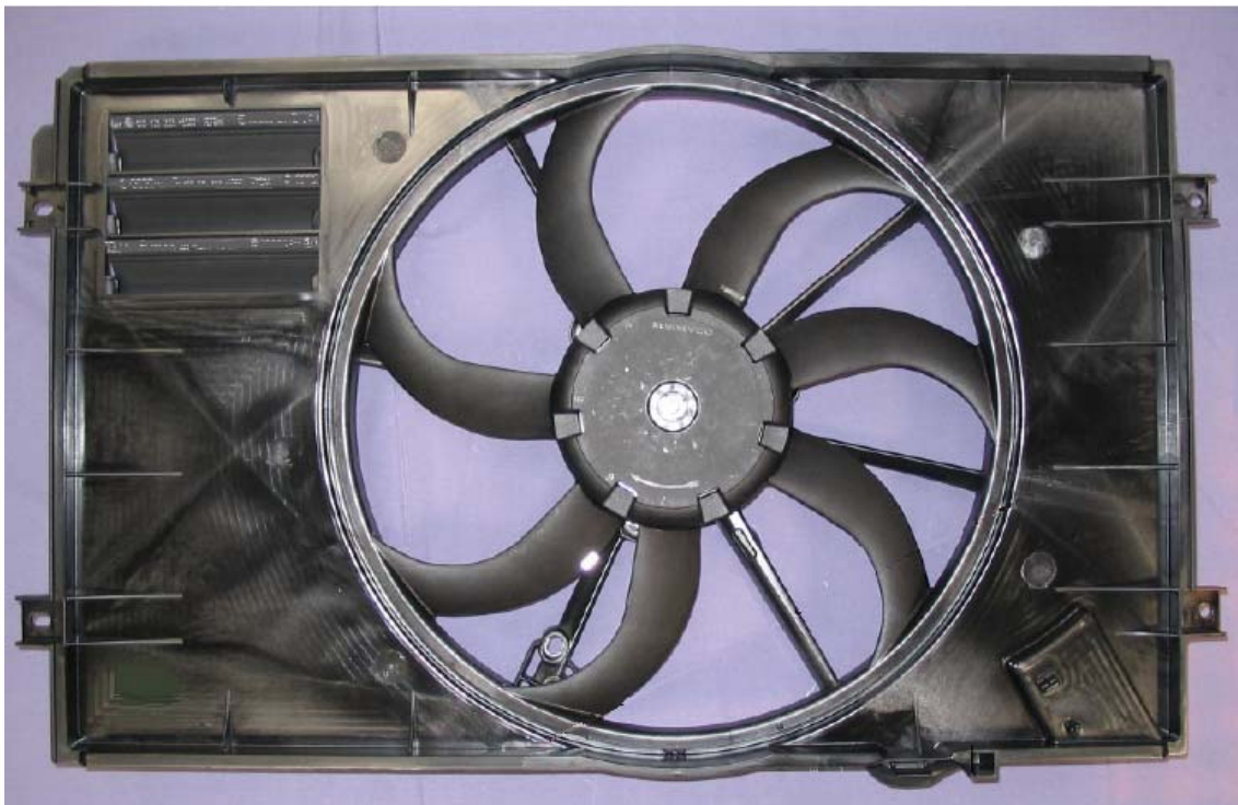
Fig.1: Fan module: fan, shroud and drive
