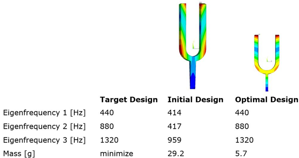
Figure 11: Comparison of the initial versus optimal design of the tuning fork.
