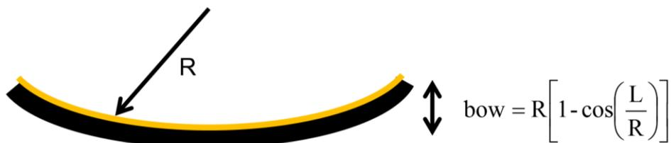
Figure 13: Curvature radius a Cu-Si bimetallic strip is the raw measured quantity. The bow is calculated afterwards and compared with simulation results.
