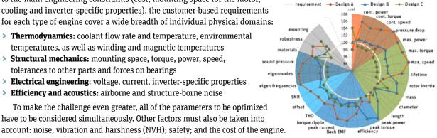
A radar chart illustrates three design concepts and how well they meet customer requirements.
