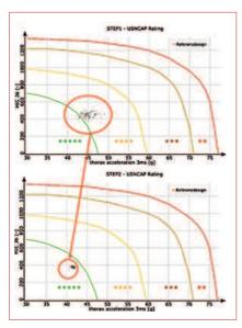
Figure 5: Visualization of robustness improvement of passive safety performance: upper diagram shows the scatter at milestone 1; lower diagram shows the scatter at final milestone of the virtual product development process
