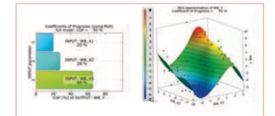
Figure 4: Coefficient of Prognosis (CoP) using the Metamodel of Optimal Prognosis (MoP) to quantify the input variable contribution to the response variable variation
