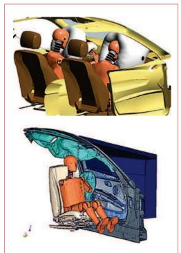
Figure 6: For passive safety applications multi body as well finite element models are used in robustness evaluation
