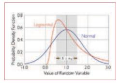
Figure 1: Normal versus Lognormal distribution, the figure visualizes that both distributions may have the same mean and standard variation but very different probability in the tails
