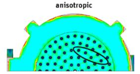
Comparison between isotropic and anisotropic elastoplastic material models. Anisotropy has a major impact on plastic strain forecast.
