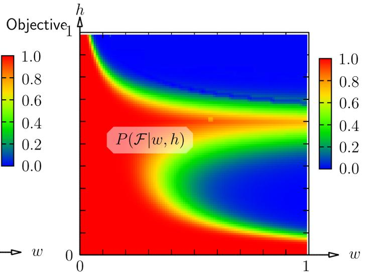
Figure 12: Failure probability depending on  $h$  and  $w$ .
