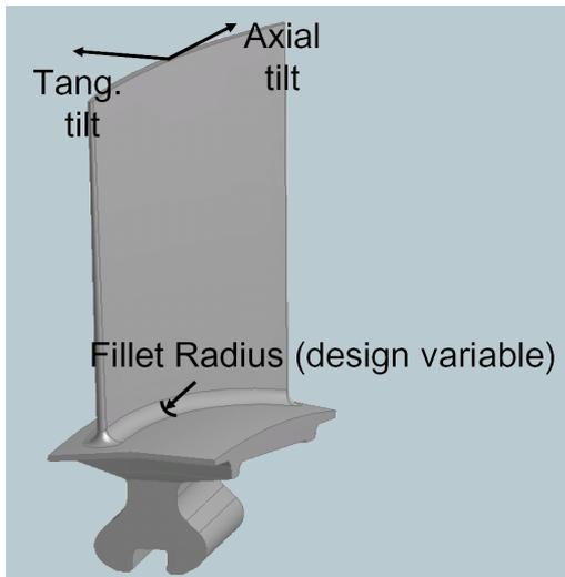
Figure 5: Turbine blade with random variables tangential and axial leaning and the design parameter fillet radius.
