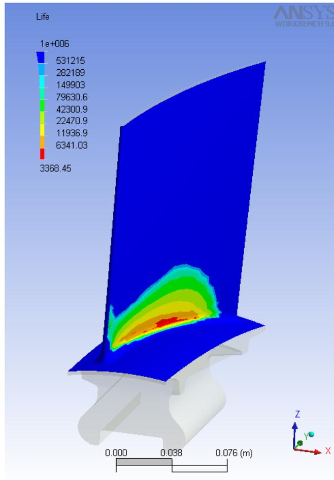
Figure 4: Turbine blade with rotational velocity and cycle fatigue life.
