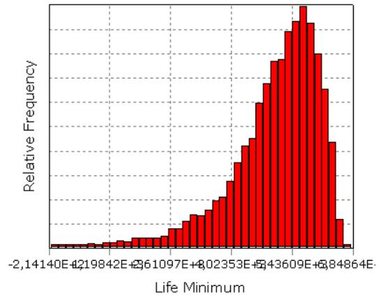
Figure 6: Probability density function of the fatigue life response.
