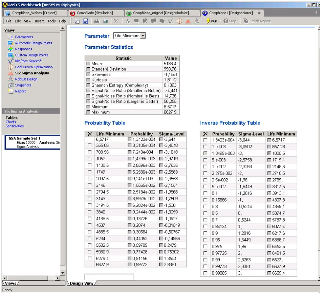
Figure 9: Example of the postprocessing of the robust design optimization using ANSYS DesignExplorer.
