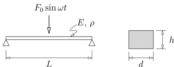
Figure 10: Beam with rectangular cross section
