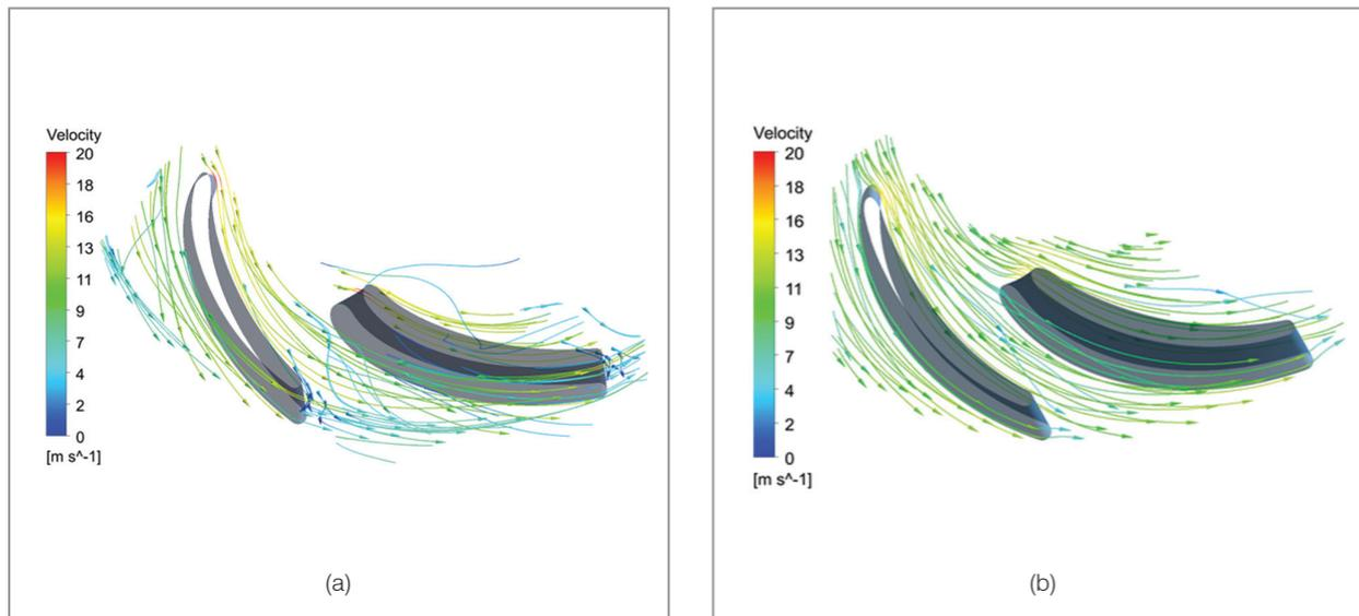
Figure 7. Velocity streamlines for (a) initial design, (b) optimized design
