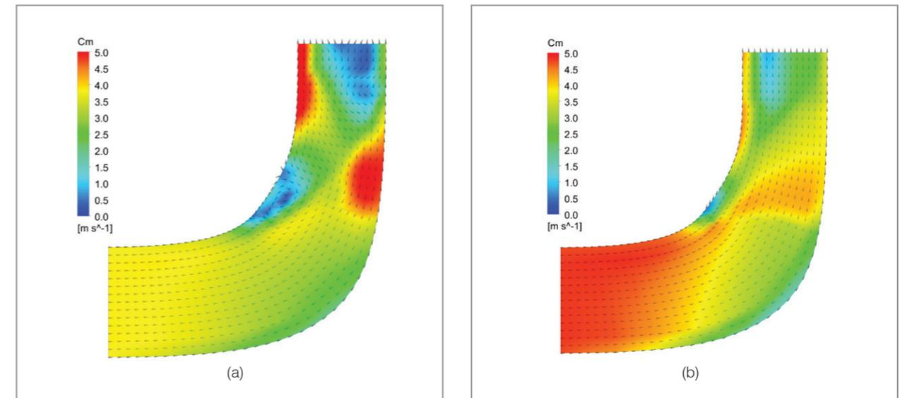
Figure 9. Meridional velocity (a) initial design (b) optimized design
