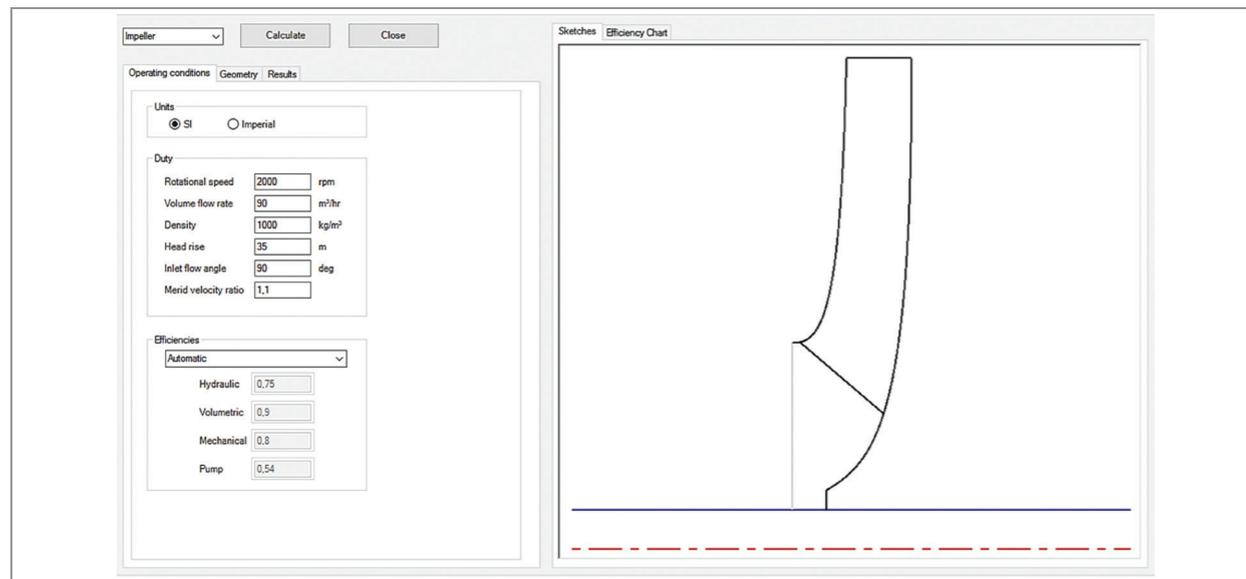
Figure 2. Input design parameters in Vista CPD
