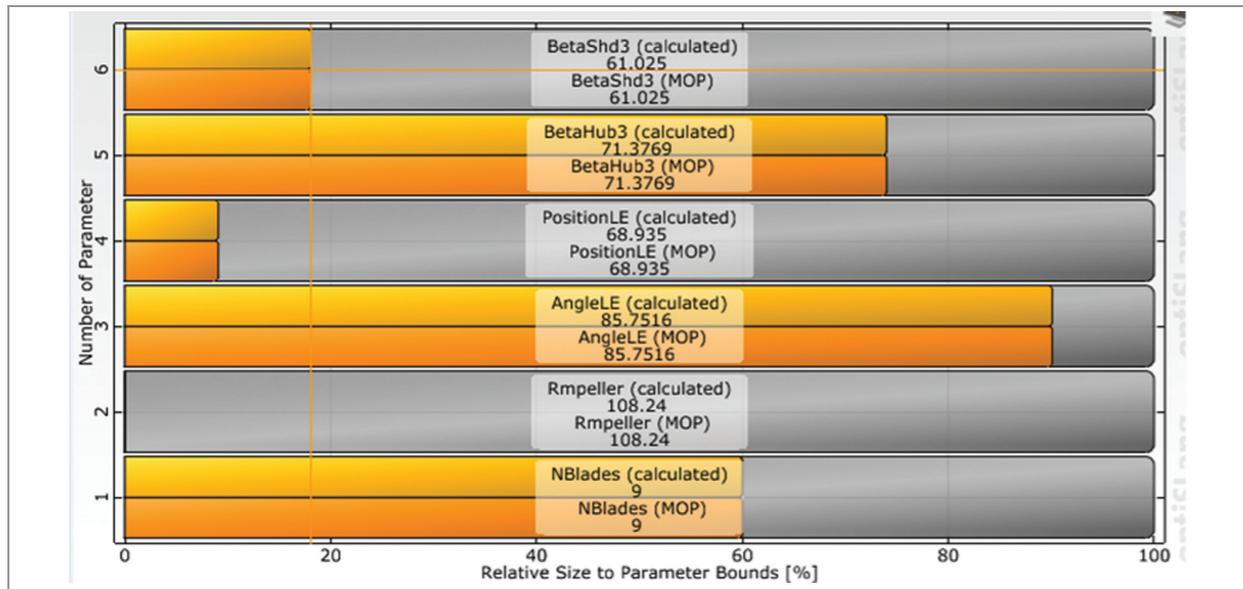
Figure 6. Values of optimized design parameters
