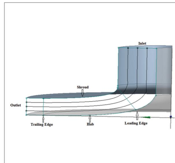
Figure 3. Meridional view of the impeller
