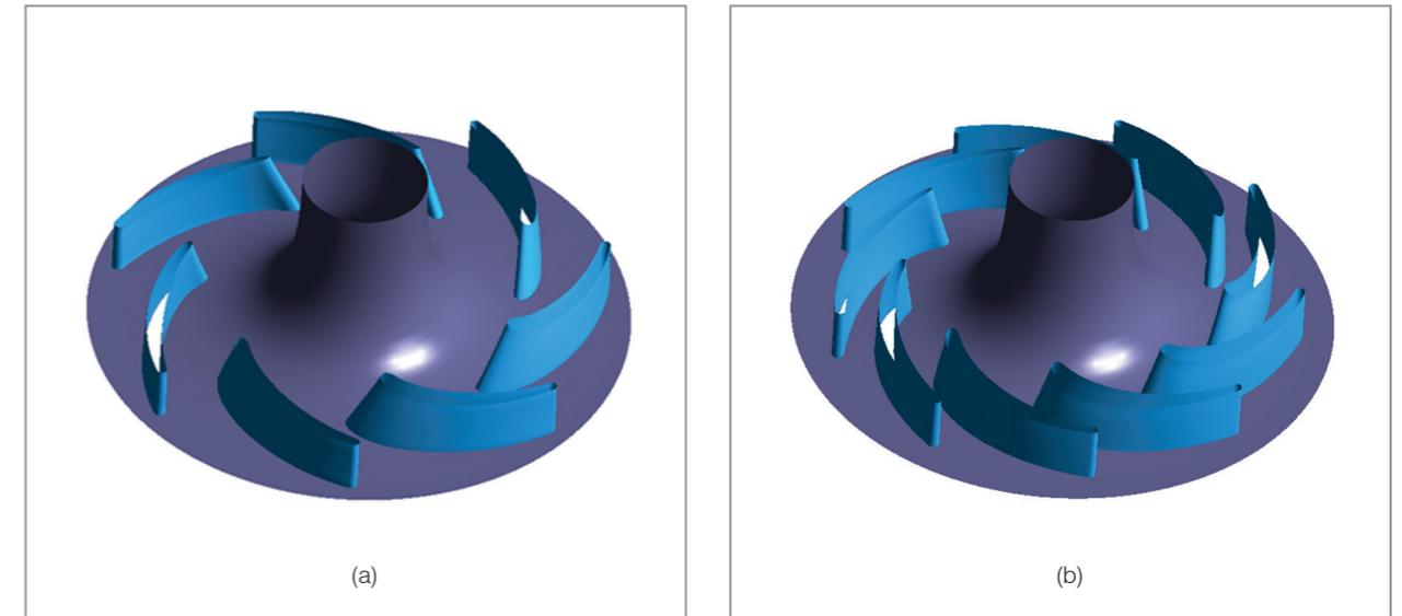
Figure 8. 3-D Models of the impeller (a) initial design (b) optimized design
