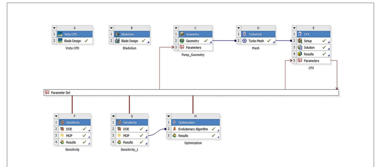
Figure 1. Optimization process flowchart
