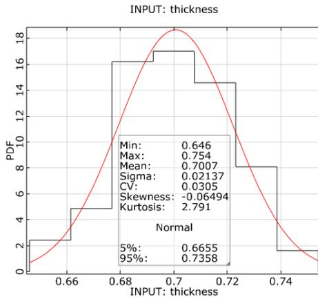
**Figure 11: Histogram sheet metal thickness**
