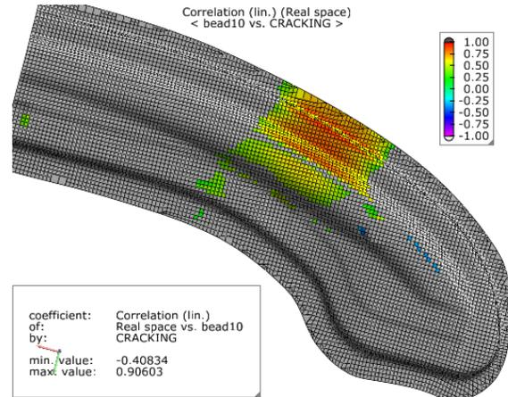
Figure 9: coefficient of correlation of force bead 10 to FLD cracking criteria
