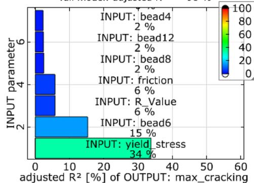
**Figure 14: CoD to maximum FLD\_cracking value**
