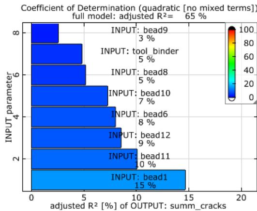
Figure 8: CoD for the sum of violating cracks
