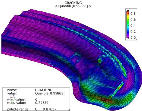
**Figure 19:** 3-sigma-value per element FLD\_cracking value robustness evaluation design\_78\_68
