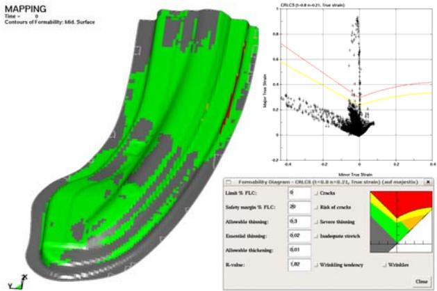
Figure 2: FLD plot and diagram of the start design
