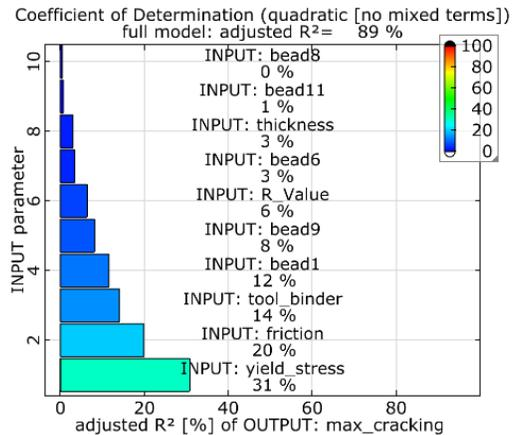
Figure 18: CoD to maximum FLD\_cracking value
