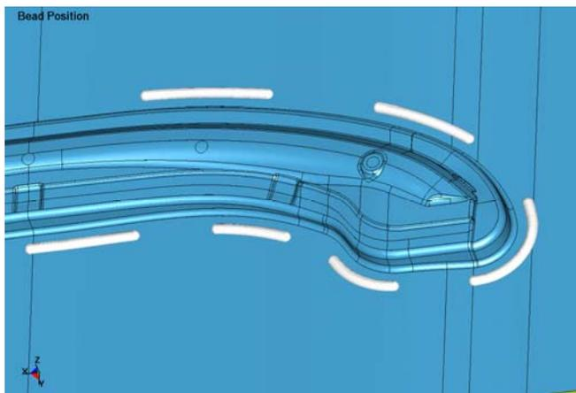
Figure 3: Positioning of the beads
