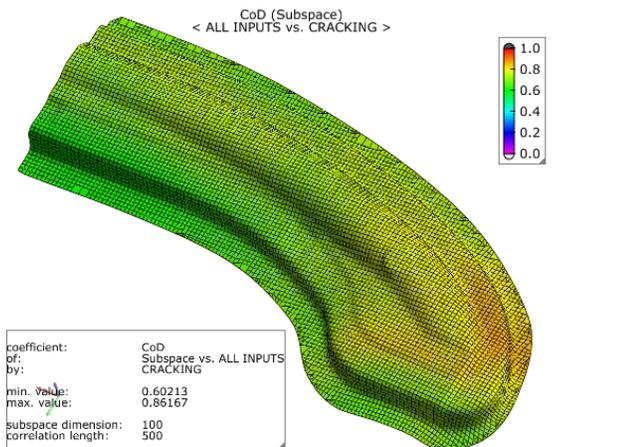
Figure 7: CoD of all inputs to FLD\_cracking criteria
