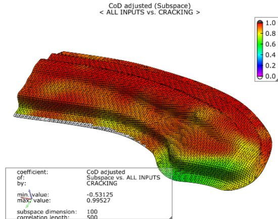
**Figure 13: coefficient of determination of all uncertainties to FLD\_cracking criteria**
