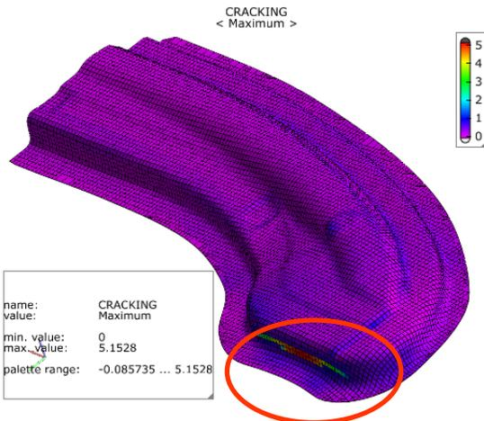
**Figure 12: maxima per element FLD\_crack value robustness evaluation design\_78**
