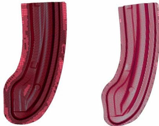
**Figure 1: left – mesh adter forming simulation
