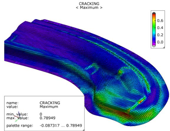
Figure 17: maxima per element FLD\_cracking value robustness evaluation design\_78\_68
