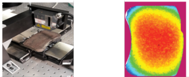
Figure 2: Measurement of a single worn brake pad surface.
