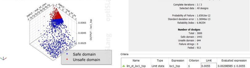
Algorithm using MOP detects with only 3000 runs very low probability of failure:  $1.7 * 10^{-12}$
