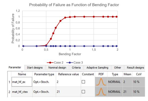
Specific design with mean E, CTE const.; Gaussian distribution; CoV 10%; bending factor varying from 0 to 2; limit level loc1\_top = 0.0055
