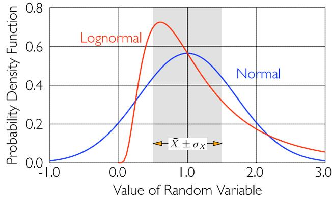
Figure 5: Normal and log-normal probability density functions.
