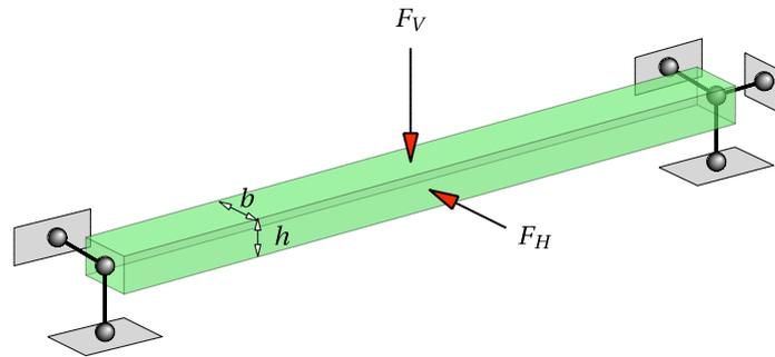
Figure 9: Beam with rectangular cross section
