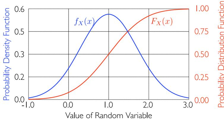
Figure 3: Schematic sketch of probability distribution and probability density functions.
