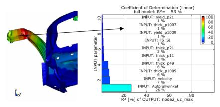
Figure 6: Measure of Determination as Indicator of the Stability Problem
