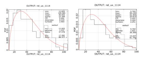
Figure 2: Histogram of the Intrusion at Node 1114, left: 84 Scattering Inputs, right: 15 Scattering Inputs
