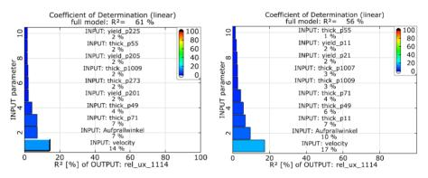
Figure 3: Measure of Determination of Intrusion at Node 1114, left: 84 Scattering Inputs, right: 15 Scattering Inputs
