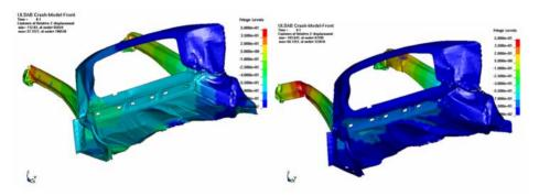
Figure 5: left: Design with Minimal Cowl Intrusion, right: Design with Maximal Cowl Intrusion
