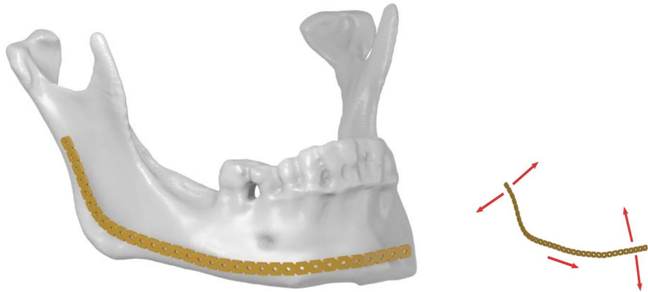
The shape of plate can be described by parameters and used in an optimization to find the best match between plate and bone surface
