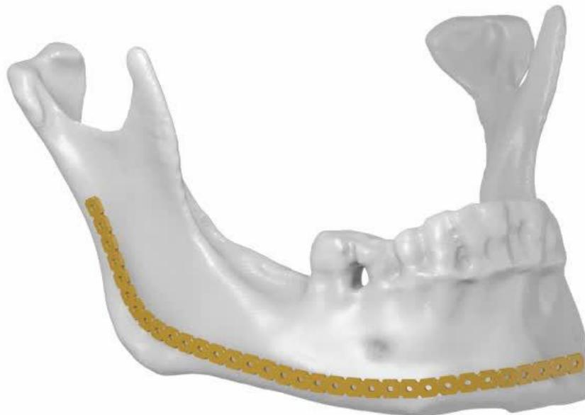
Shape of plate can be optimized to find the best match between plate and bone surface
