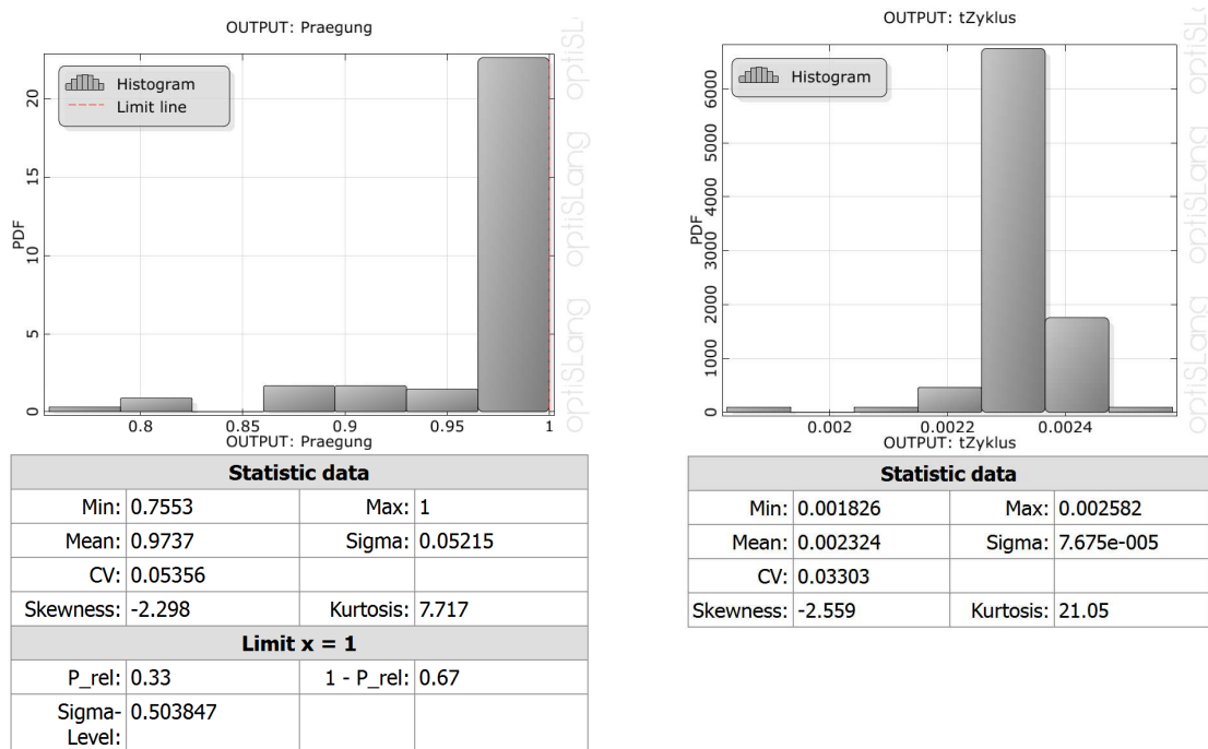
Figure 6: Statistical data of the embossing (left) and the cycle time (right) at the deterministic optimum
