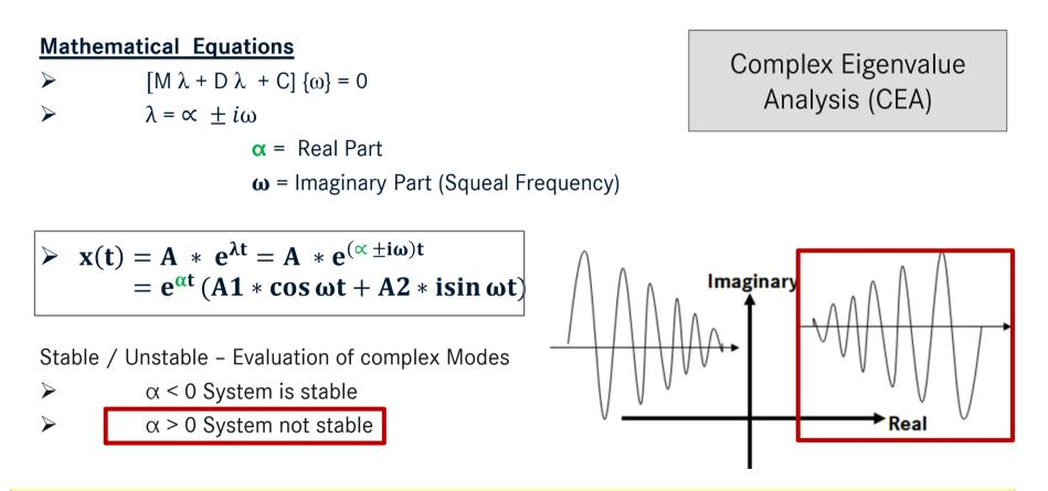
Positive  $\alpha$  indicates a system behavior with an increasing amplitude of the brake oscillation
