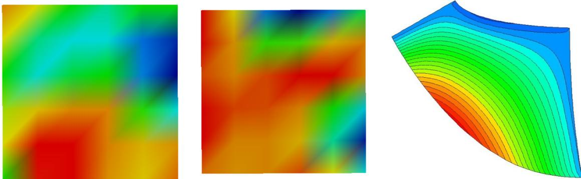
**Fig. 3** Example of random fields' realizations (left), correlated thickness distributions (right)
