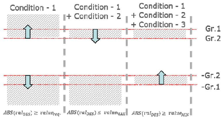
**Fig. 8** Example of “two belts filter”
