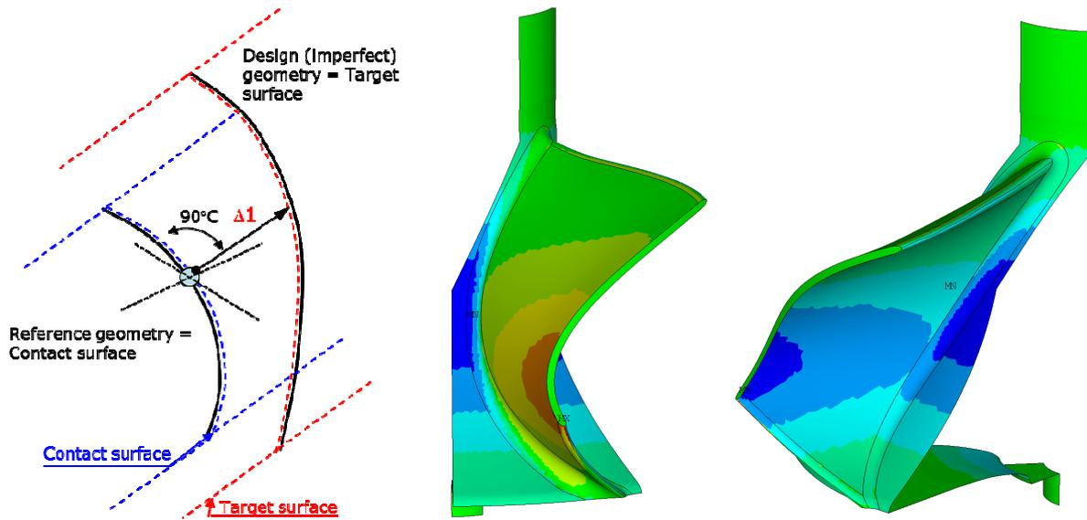
Fig. 1 Example of external surfaces deviations on the blade and hub body
