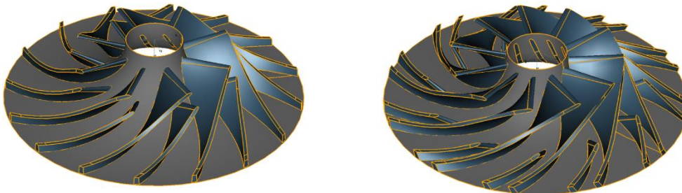
Figure 6 Impeller geometries (left: initial, right: optimized design) created by CFTurbo®.
