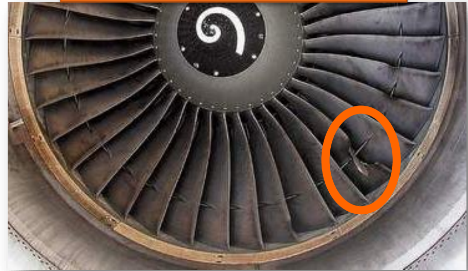
Rotor Damage at Blade x
