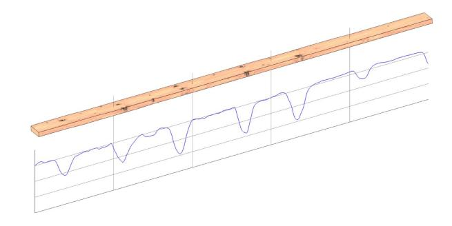
• Variation of mass density, knots & moisture content lead to material property fluctuations in wooden boards
