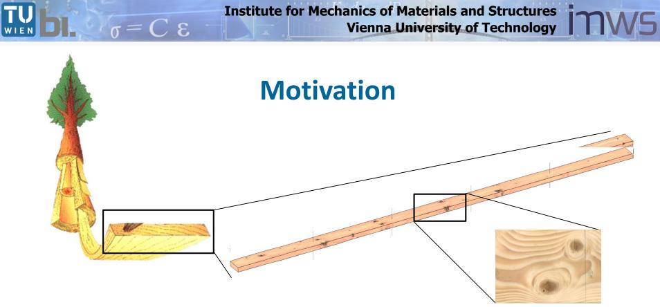
• Variation of mass density, knots & moisture content lead to material property fluctuations in wooden boards
