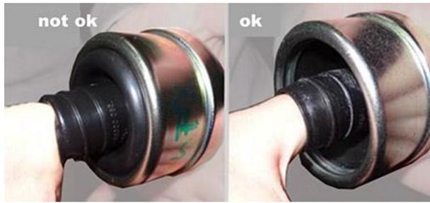
Fig. 2: "S-punch shaped" deformation (left) and optimal rolling off behavior (right) of the rubber boot
