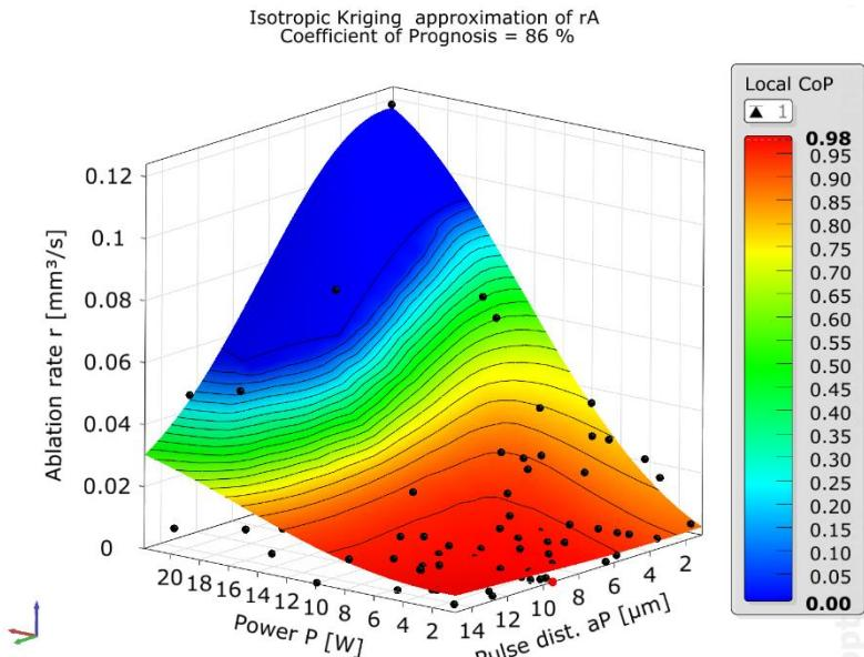
→ Good roughness model due to large value range ( $R_a = 0,4 \dots 3,8 \mu\text{m}$ )
