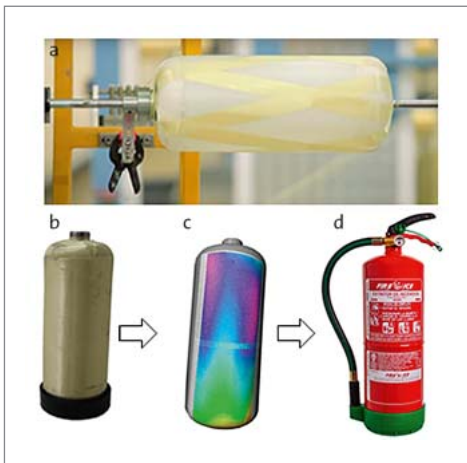
Fig. 1: a-Filament winding technique b-COPV / c-Digital image correlation for Random Fields / d-Fire extinguisher
