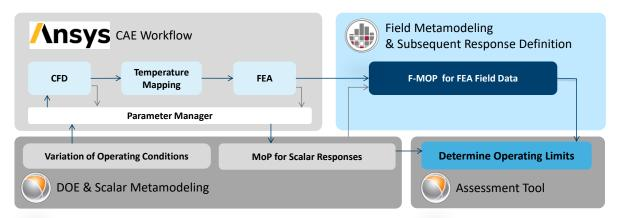
Figure 5: Example of Rheinmetall Automotive Workflow for subsequent Response Definition
