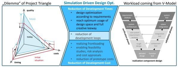
Figure 1: Motivation for simulation driven design optimization
