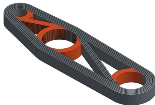
Figure 2: Half of the composite mountain bike rocker with its different composite paths and plastic areas
