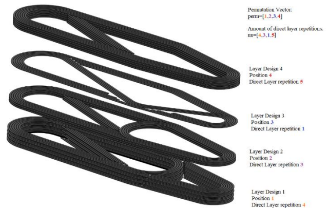
Figure 4: Exemplary layer sequence for perm[1,2,3,4] and nn=[4,3,1,5]
