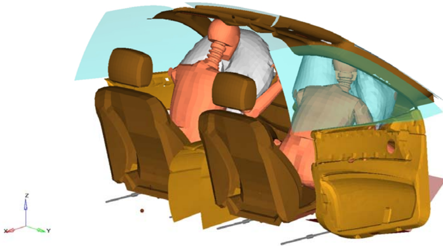
Figure 2: Simulation Passenger Safety Load Case FMVSS 208
