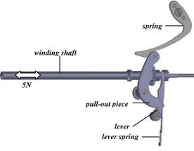
Fig. 1: Set time mechanism
