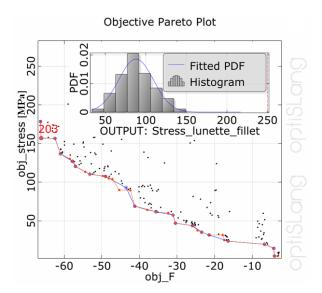
Fig. 6: Result of the Pareto optimization in optiSlang. The probability density function for the maximum stress in the watch-case obtained with a robustness analysis for design 203 has been inserted.
