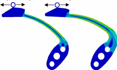
Fig.2: Spring initial shape (left) and tuned shape (right). The pin of the pull-out piece is at the force inversion position where stresses reach their maximum. The positioning and angle of the two flat contact faces of the spring determine the pull and push forces.
