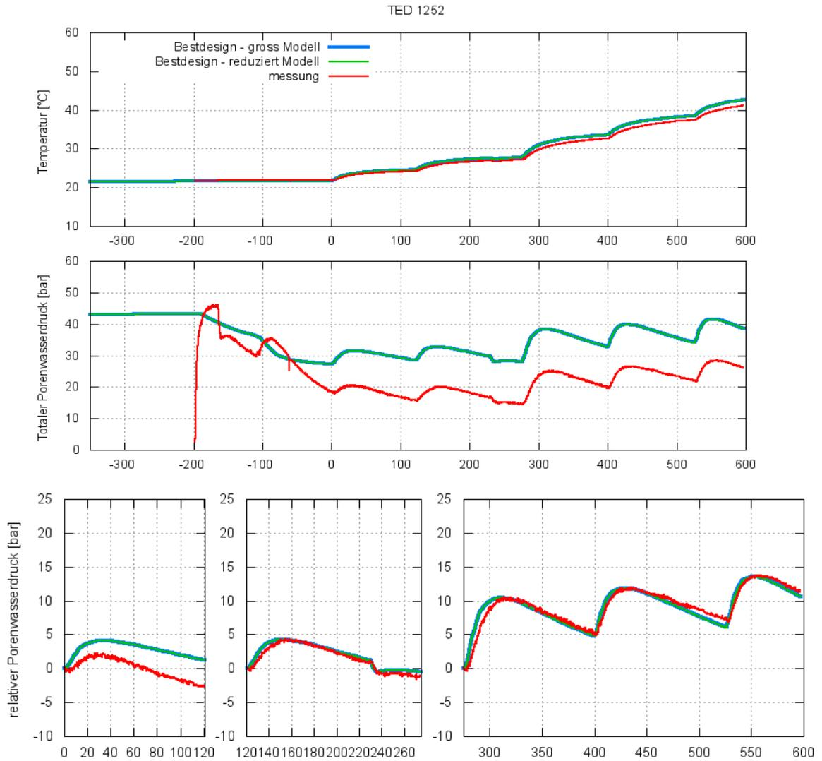
Figure 8: Comparison of simulation vs. measurement at point 1252 after the parameter identification. Top: temperature curve, middle: total pore water pressure, bottom: relative pore water pressure of the three heating periods
