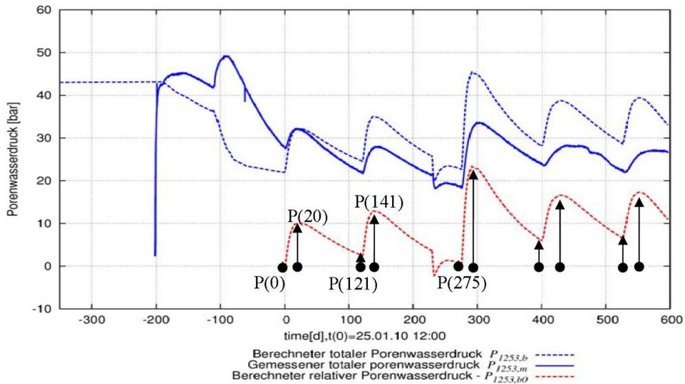
Figure 3: Relative pore water pressures for parameter identification
