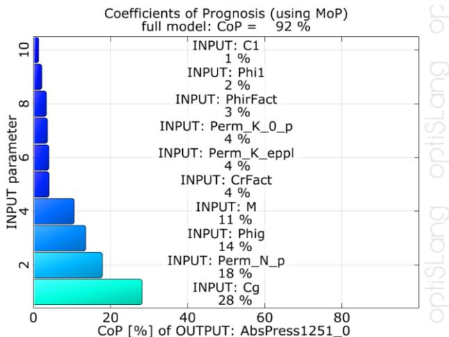
Figure 4: CoP relative pore pressure at time  $t = 0$ , the measuring point in 1251
