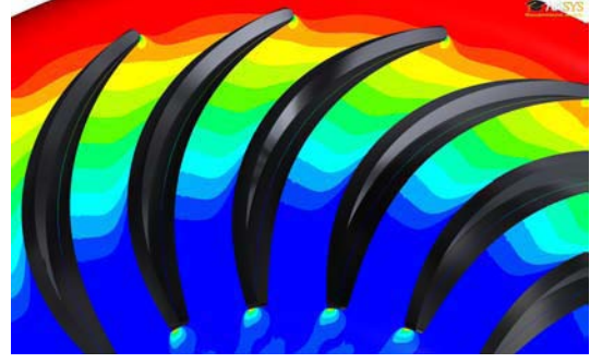
Figure 13: Flow angle of the optimized design at the returnvane blades with a much more uniform flow
