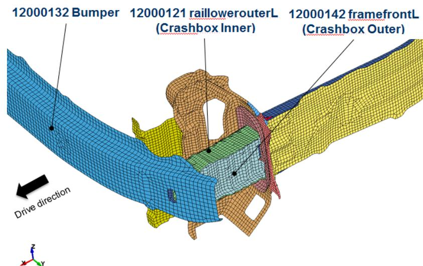
Figure 3 Relevant TOYOTA Yaris front end parts
