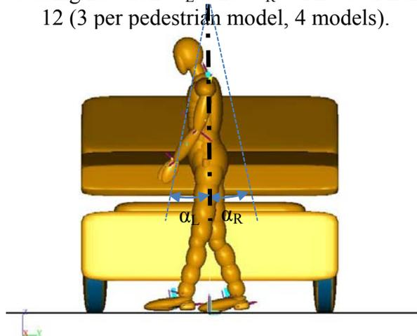
Figure 7 MADYMO set-up showing angle between legs (gait)
