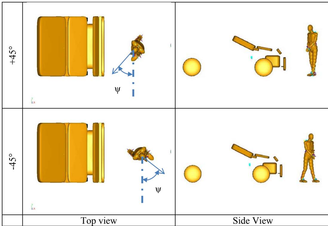
Figure 6 Pedestrian simulation input set up (Angle with car  $-\psi$ )
