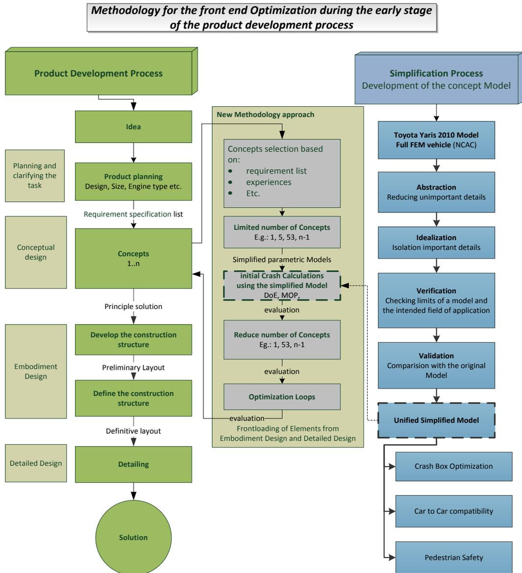
Figure 1: Methodology for the front end Optimization during the early stage of the product development process
