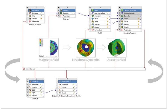
Fig. 4: Full parameterized optimization environment with optiSLang inside ANSYS Workbench
