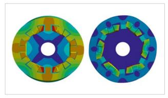
Fig. 2: Normal modes of outer parts of a motor
