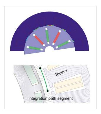
Fig. 3: Co-energy distribution inside the air gap and stator of a synchronous machine with permanent magnets and reduced force integration pathor
