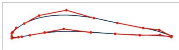
Fig. 7: The definition of blade profile geometry (blue) using control points (red)
