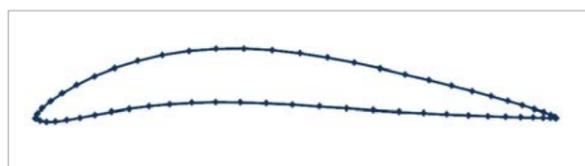
Fig. 6: Definition of blade profile geometry using data points
