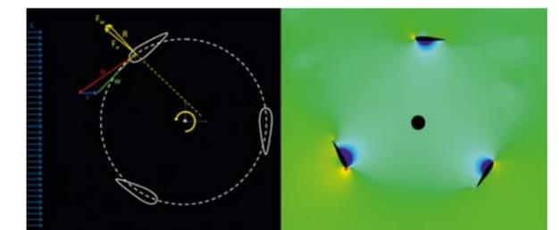
Fig.4: The working principle of a vertical axis wind turbine (left) velocity vectors and pressure distribution on blades (right)
