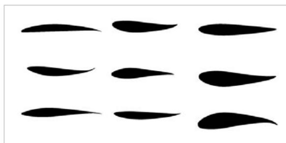
Fig. 9: A selection of parameter-based profiles
