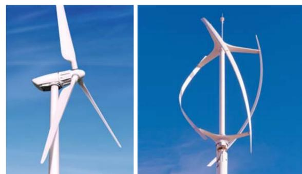
Fig. 1: Left - horizontal axis wind turbine; right - vertical axis wind turbine
