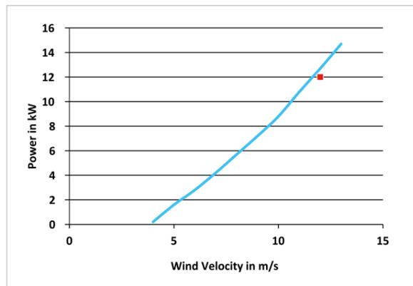
Fig. 16b: Validation of plot by comparison with measured data from an existing turbine near Uppsala, Sweden
