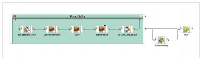
Fig. 4: optiSLang workflow of an automized sensitivity study for a Rocky DEM simulation
