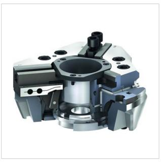
Fig. 6: The axially displaceable piston transmits the force to the base jaws and generates a radial jaw movement synchronous to the axis of rotation
