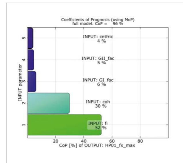
Fig. 6: Coefficients of prognosis – lowest hammer position
