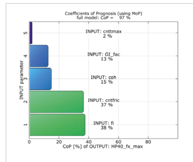
Figure 8: Coefficients of prognosis – highest hammer position
