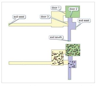
Fig. 1: Room geometry (top) and initial distribution of occupants (bottom)
