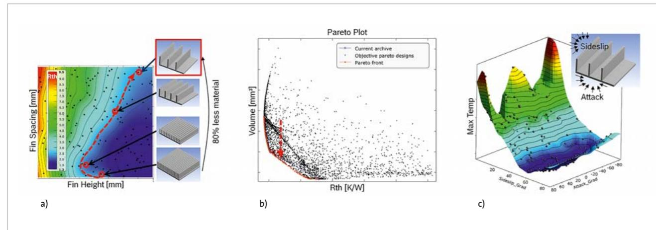
Figure 2: a)  $R_{th}$  value of cooler with fins depending on geometry with indicated isoline, b) Pareto plot depending on cooler volume and c) sensitivity analysis of air flow vector depending on maximum cooler temperature
