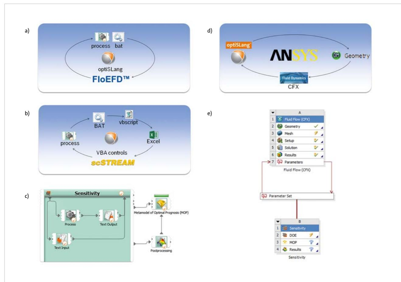
Figure 1: Implementation of workflows. a) - c) standalone optiSLang, d), e) optiSLang inside ANSYS Workbench.
