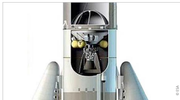
Fig. 1: Upper stage Midlife Evolution (ME) of the launcher Ariane 5
